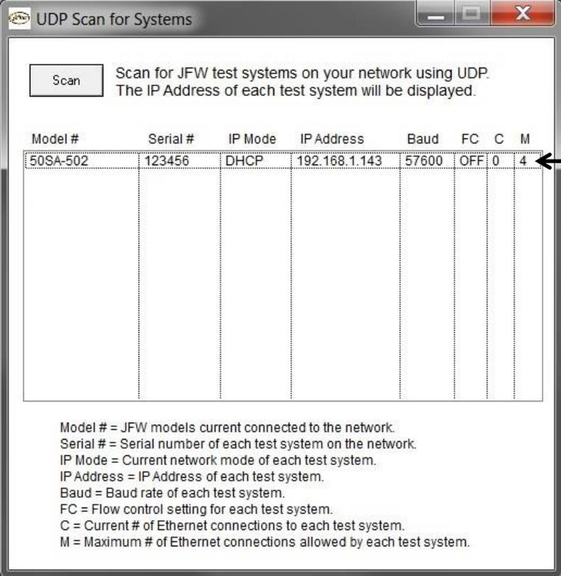
The screenshot shows a window titled "UDP Scan for Systems" with a "Scan" button and a description: "Scan for JFW test systems on your network using UDP. The IP Address of each test system will be displayed." Below this is a table with the following data:
