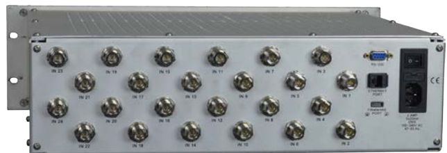
24 attenuators 3RU 19" rack enclosure No front panel control N inputs on rear / SMA outputs on front
