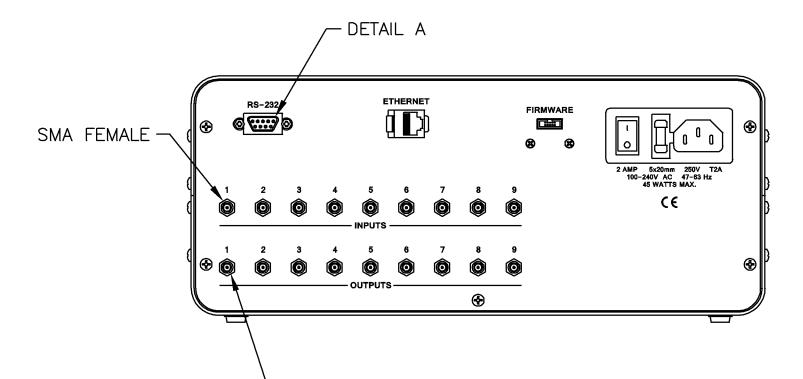
THE NUMBER OF SMA DEPENDS ON THE MODEL NUMBER "-04" MODELS W/ 4 ATTENUATORS HAVE 8 SMA FEMALE "-06" MODELS W/ 6 ATTENUATORS HAVE 12 SMA FEMALE "-09" MODELS W/ 9 ATTENUATORS HAVE 18 SMA FEMALE
